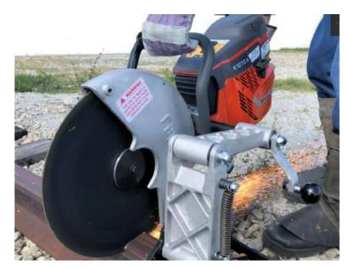
The Ultra Kut III uses the Husqvarna K1270R power head, which is specially designed for heavy-duty use.
